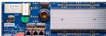
RS485 Communication between battery and inverters Band rate:9600ps RS485 Interface Communication between parallel packs or BMS and PC Band rate:9600ps
